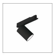
Spot 31, directional spotlight, light control with lens, of PMMA, LED rated luminous flux: 5.040lm, light colour: 940, with 3-phase adapter, mains connection: 220..240V, AC, 50/60Hz, of aluminium, jet black (RAL 9005), length: 213mm, diameter: 90mm, protection rating (complete): IP20, insulation class (complete): insulation class I (protective earthing), certification: CE, impact resistance: IK02, permissible ambient temperature for indoor applications: -20..+40°C, packaging unit: 1 piece
