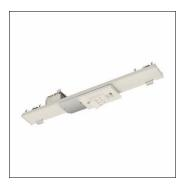
Licross® Trunking, rail insert, with plug, 6-pole, with phase selection, mains connection: 230V, AC, 50Hz, adapter, of sheet steel, coil coated, white, for speaker TOA BS-1034EN, length: 500mm, width: 64mm, height: 102mm, speaker adapter insert, protection rating (complete): IP20, insulation class (complete): insulation class I (protective earthing), certification: CE, UKCA, packaging unit: 1 piece
