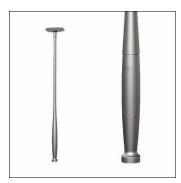
mast, mast, conical round, of aluminium, coated, Siteco® metallic grey (DB 702S), height: 4.0m, spigot size: 76mm (post-top), planted section: h= 800mm / Ø= 140mm, standard: DIN EN 40, packaging unit: 1 piece
