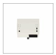
SITECO Connect 21-Ocontroller, master, central control, dimmable, installation type: recessed, installation location: in an electrical distributor, of plastic, part units: 9 part units, protection rating (complete): IP20, insulation class (complete): insulation class I (protective earthing), certification: CE, voltage: 100..240V, voltage type: AC, 1 x network connector Ethernet, 4 x DALI, 4 x relay contact, packaging unit: 1 piece
