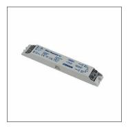
SITECO Connectrepeater, master, central control, dimmable, installation type: recessed, installation location: in the luminaire, of plastic, protection rating (complete): IP20, insulation class (complete): insulation class I (protective earthing), certification: CE, voltage: 100...240V, voltage type: AC, 1 x DALI, 1 x TouchDim input, 1 x DALI broadcast, packaging unit: 1 piece
