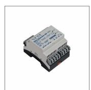
SITECO Connectrepeater, master, central control, dimmable, installation type: recessed, installation location: in an electrical distributor, of plastic, part units: 4 part units, protection rating (complete): IP20, insulation class (complete): insulation class I (protective earthing), certification: CE, voltage: 100..240V, voltage type: AC, 2 x DALI, 1 x TouchDim input, 1 x DALI broadcast, packaging unit: 1 piece
