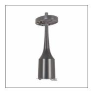
electrics components group, for Module 540 iQ, gear tray, control gear: ECG iQ, LED luminous flux: 1.510 lm, colour temperature: 3000K, with terminal, 6-pole, max. 2.5mm², mains connection: 230..240V, AC, 50/60Hz, start of lifetime: 11 W, end of service life: 11 W, reduction: 5 W, primary light characteristic: strongly asymmetric, width: 190 mm, height: 514mm, insulation class (complete): insulation class II (safety insulation), certification: CE, ENEC, VDF
