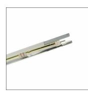
Modario<sup>®</sup>, trunking rail, of sheet steel, coated, pure white, 10x system unit 299mm 10-core and 2x system unit 1495mm 2-core, length: 2.990 mm, width: 58 mm, height: 43mm, through-wiring: 12x 2.5mm<sup>2</sup>, with terminal, 10+2-pole, max. 2.5mm<sup>2</sup>, protection rating (complete): for IP20 protection rating, insulation class (complete): insulation class I (protective earthing), certification: CE, ENEC, VDE, standard: EN 60598, packaging unit: 1 piece
