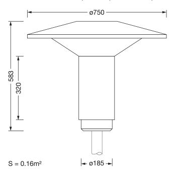
It is mandatory that the assembly instructions must be observed when planning and installing the electrical installation (to be found at www.siteco.de) Tolerances related to thermal, electrical and photometric data according to IEC 62722 Issued 14.06.2024 - Modifications and errors subject to change - Ensure that you always use the latest version -
