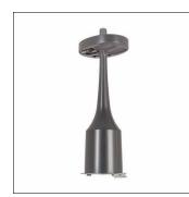
electrics components group, for Module 540 iQ, gear tray, control gear: ECG iQ, LED luminous flux: 1.510 lm, colour temperature: 2200K, with terminal, 6-pole, max. 2.5mm<sup>2</sup>, mains connection: 230..240V, AC, 50/60Hz, start of lifetime: 13 W, end of service life: 13 W, reduction: 6 W, primary light characteristic: strongly asymmetric, width: 190 mm, height: 514mm, insulation class (complete): insulation class II (safety insulation), certification: CE, ENEC, VDE
