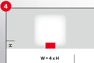
PL64 – to illuminate areas using a narrow beam spread
